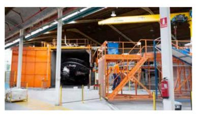
With three separate arms, this machine can load up to **65 moulds.**
