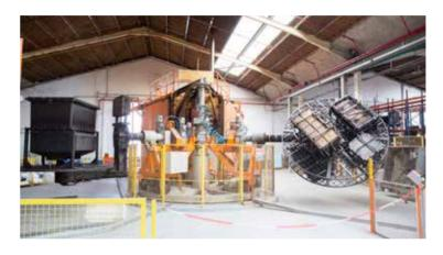
With three separate arms, this machine can load up to **24 moulds.**
